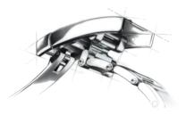
To ensure optimal comfort when wearing your watch in any circumstances, Rolex created the Easylink comfort extension link, which is available on some models. Its exclusive design, which was patented, allows the length of the bracelet to be adjusted by approximately 5 mm, without the use of tools.
